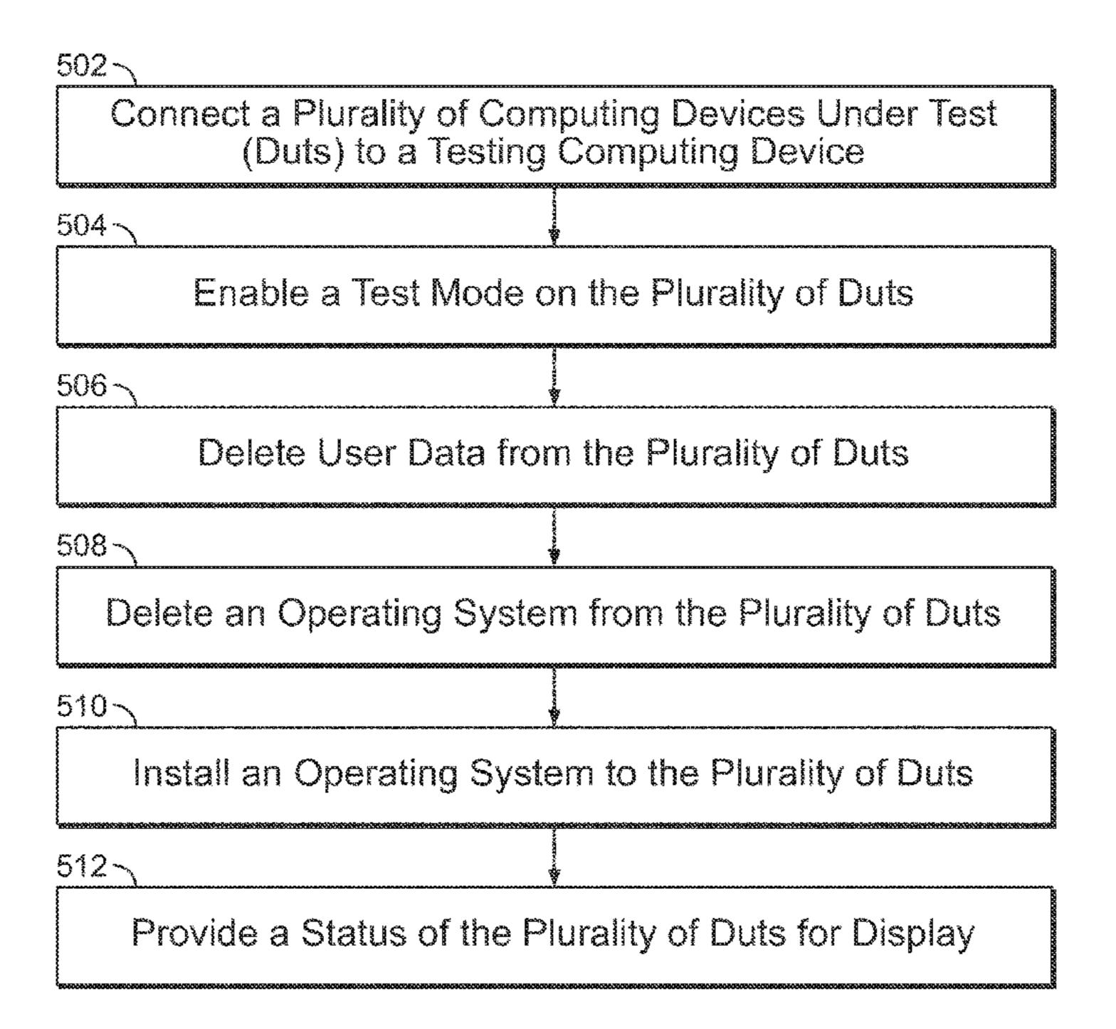
may also include a bracket that secures a monitor and a keyboard, where the monitor and keyboard are communicatively coupled to the testing computing device. The testing computing device can simultaneously service the plurality of computing devices, such as by causing the deletion of user data, the loading of software, and the testing of various functions.
