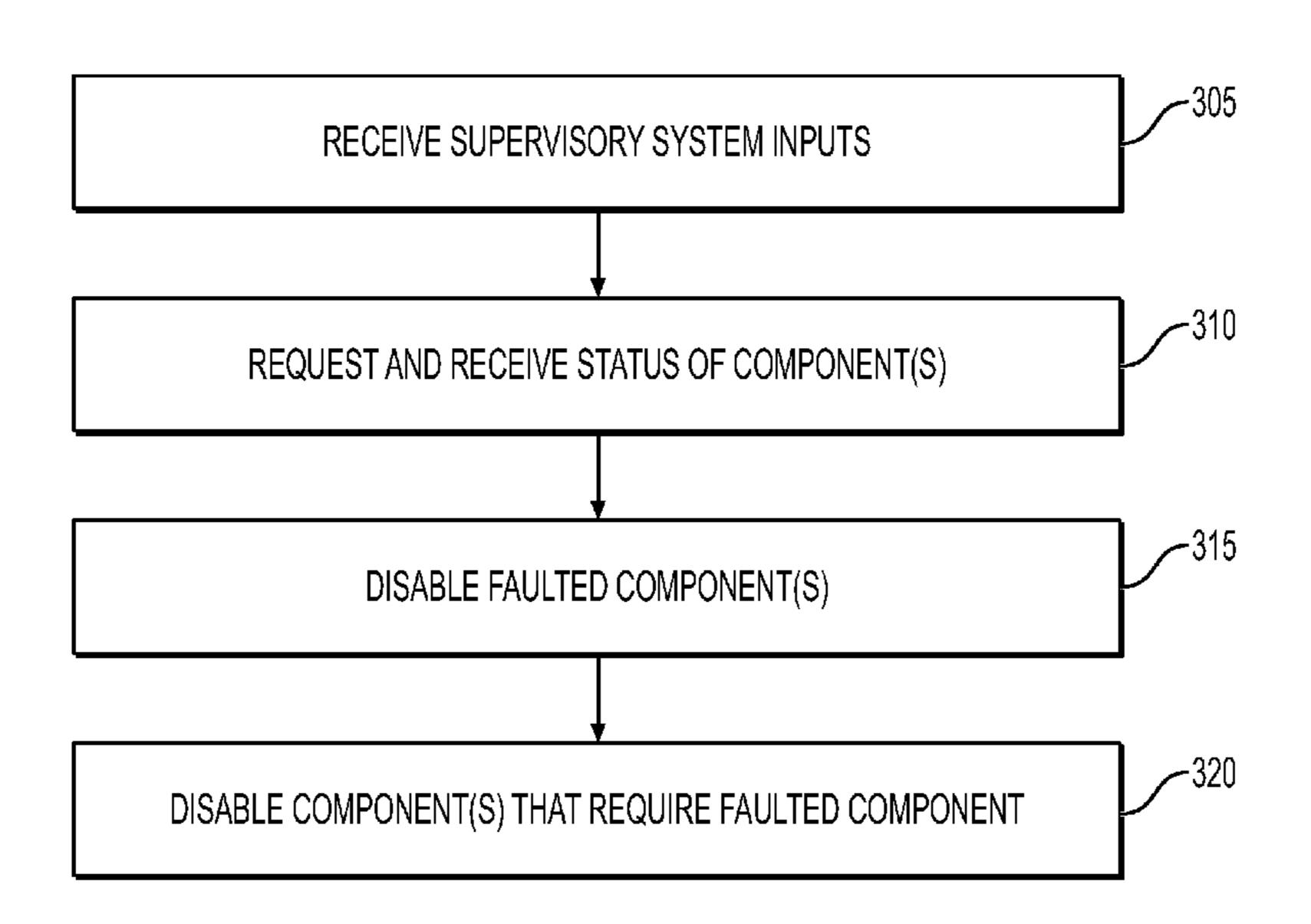
more component controllers, a status of the one or more components, and, upon receiving an indication that a status of a component, of the one or more components, is faulted, disabling the faulted component, and disabling any other components, of the one or more components, that require the faulted component for operation.
