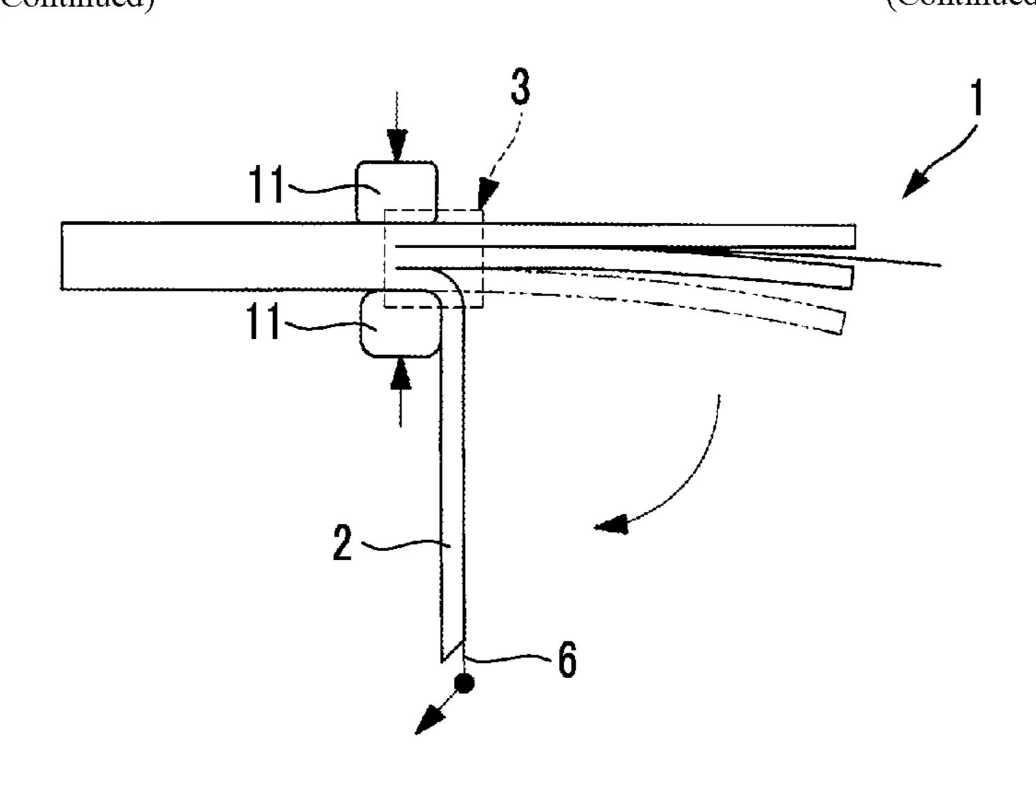
from an end edge on a bent side to the bendable portion, the laminate is divided into layers along a plate thickness direction of the laminate.
