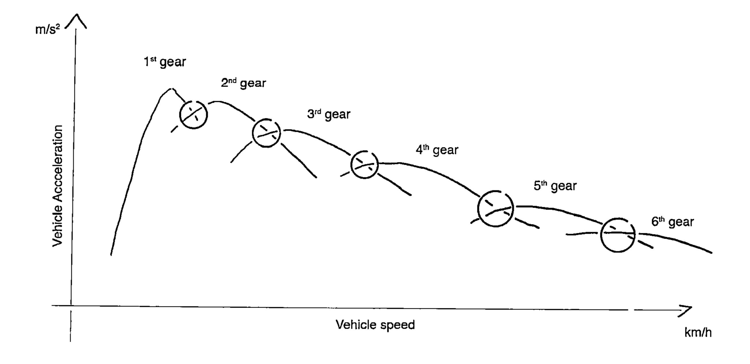
Figure 1 - Acceleration plot for each gear (1-6) vs. vehicle speed; Intersections between curves circled.
