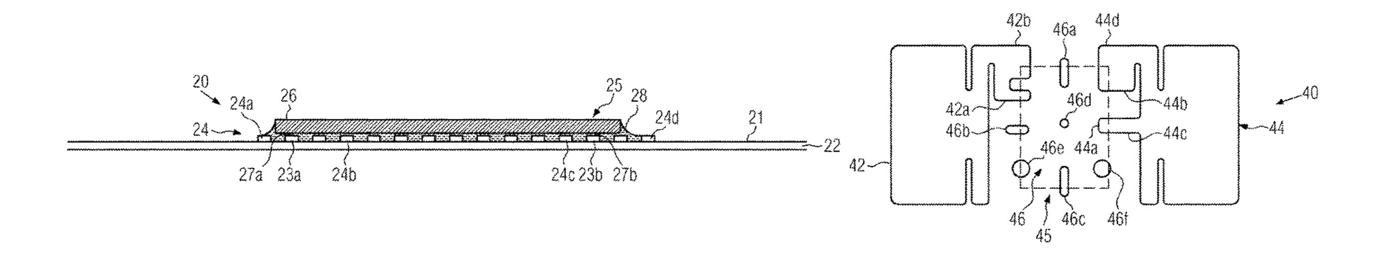
the at least one contact pad each represent a support for the chip on the prelam body substrate.
