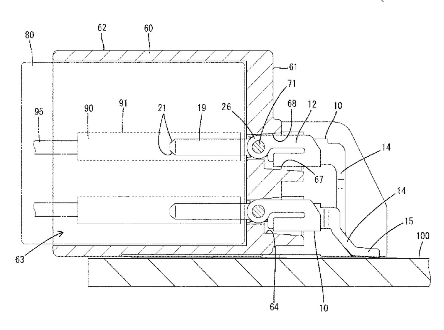
tion and the board connecting portion. The housing includes a supporting portion for rotatably supporting the terminal fitting by being engaged with the shaft portion. The terminal fitting has a center of gravity on a side closer to the board connecting portion than the shaft portion.
