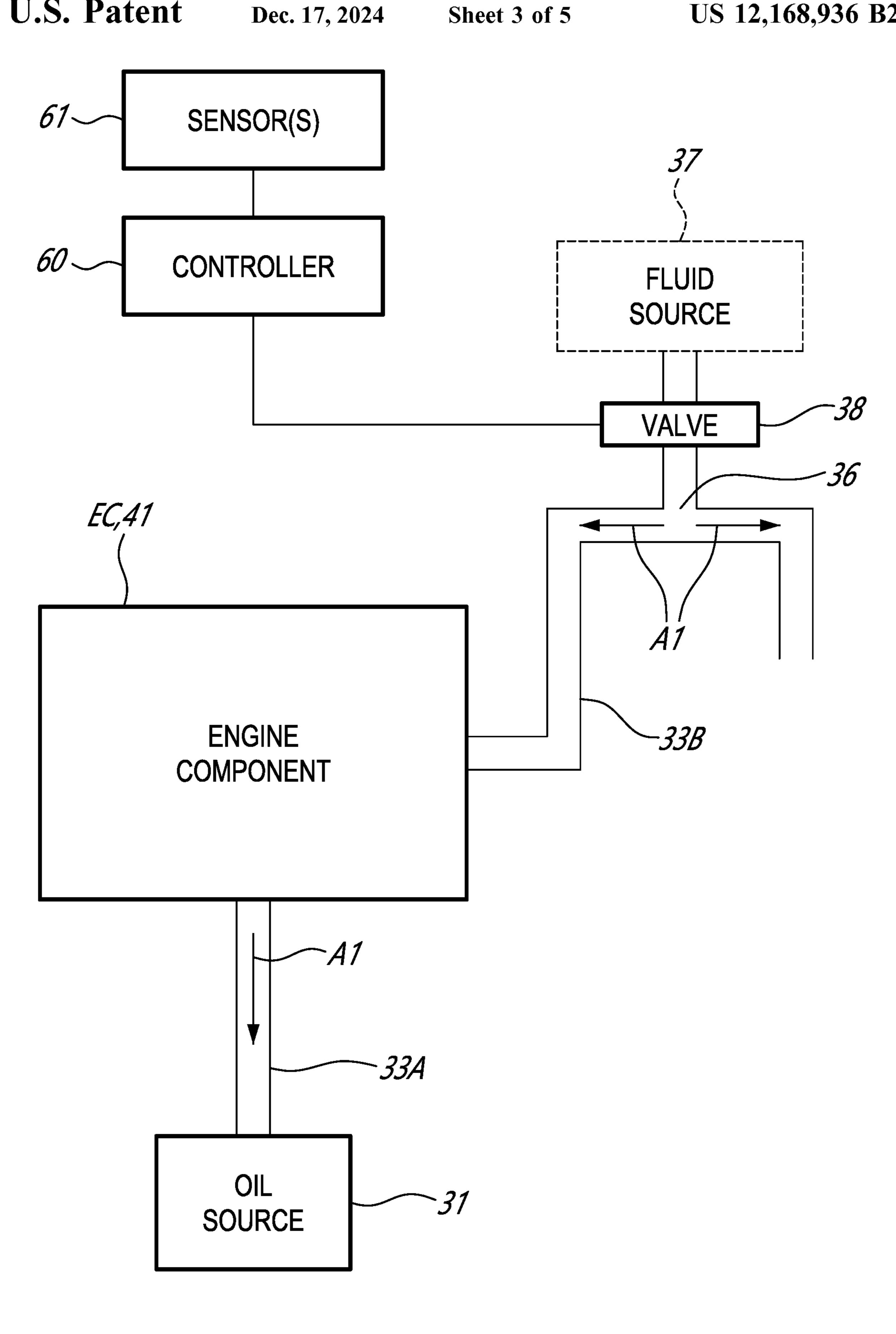
Determine that the component is subjected to a fire event, the component containing a baseline volume of the flammable fluid, the baseline volume of the flammable fluid being greater than a maximum volume of the flammable fluid for compliance with fire resistance requirements
