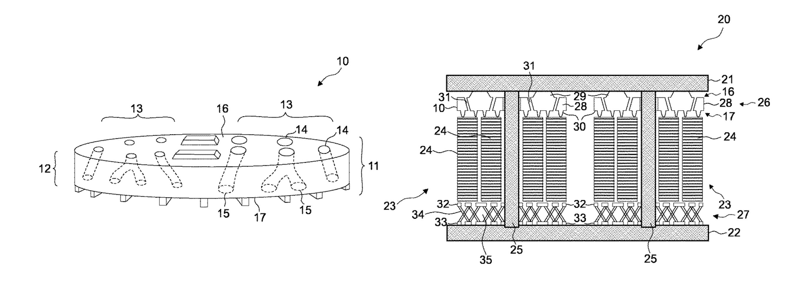
flow structure are formed as one integrated part comprising a polymer material. The integrated part comprises a plurality of orifices for passage of the liquid coolant from a first side facing the holding structure to a second side facing the at least one winding.
