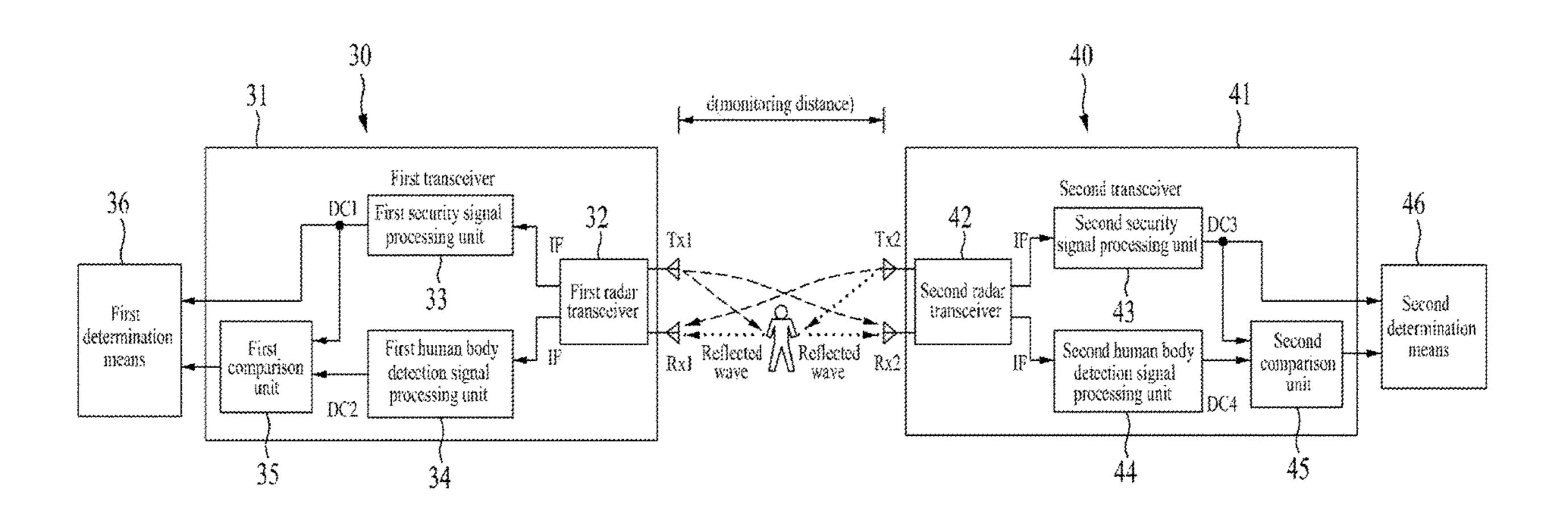
reduce the false report rate by distinguishing the false alarms or the malfunction state of the sensor.
