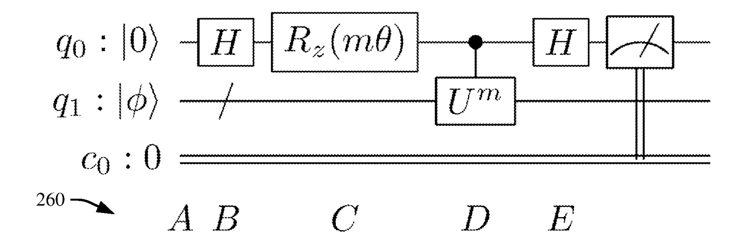
where,  $R_z(m\theta) = e^{im\theta Z/2}$  and  $U|\phi\rangle = e^{i\phi}|\phi\rangle$
