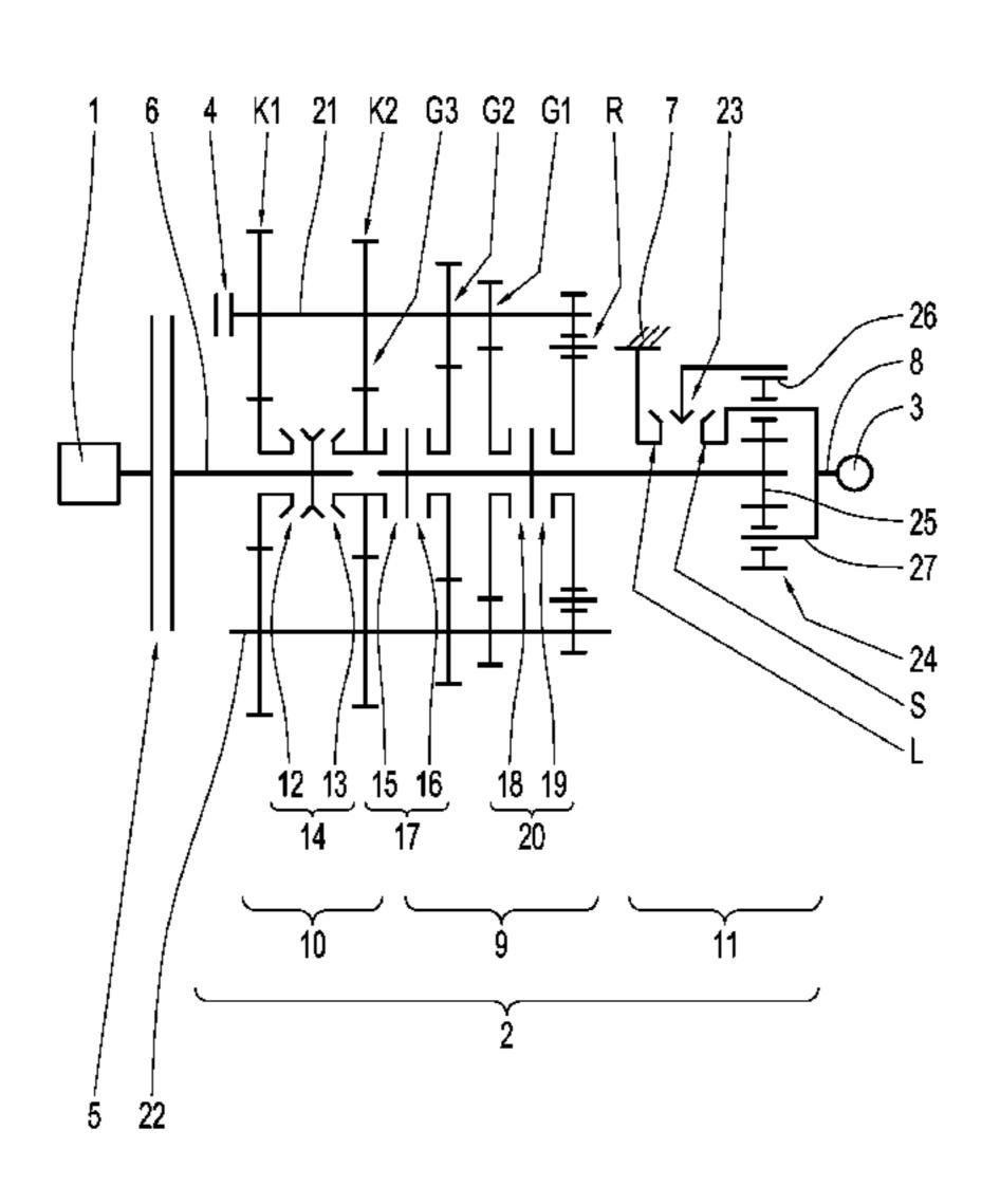
shifting program is activated. Shifting from a current gear to a target gear is carried out automatically, as a function of input rotation speed of the group transmission or as a function of rotation speed of the drive aggregate, while the disconnect clutch is closed and where the main transmission and/or the range group participate exclusively, but not the splitter group.
