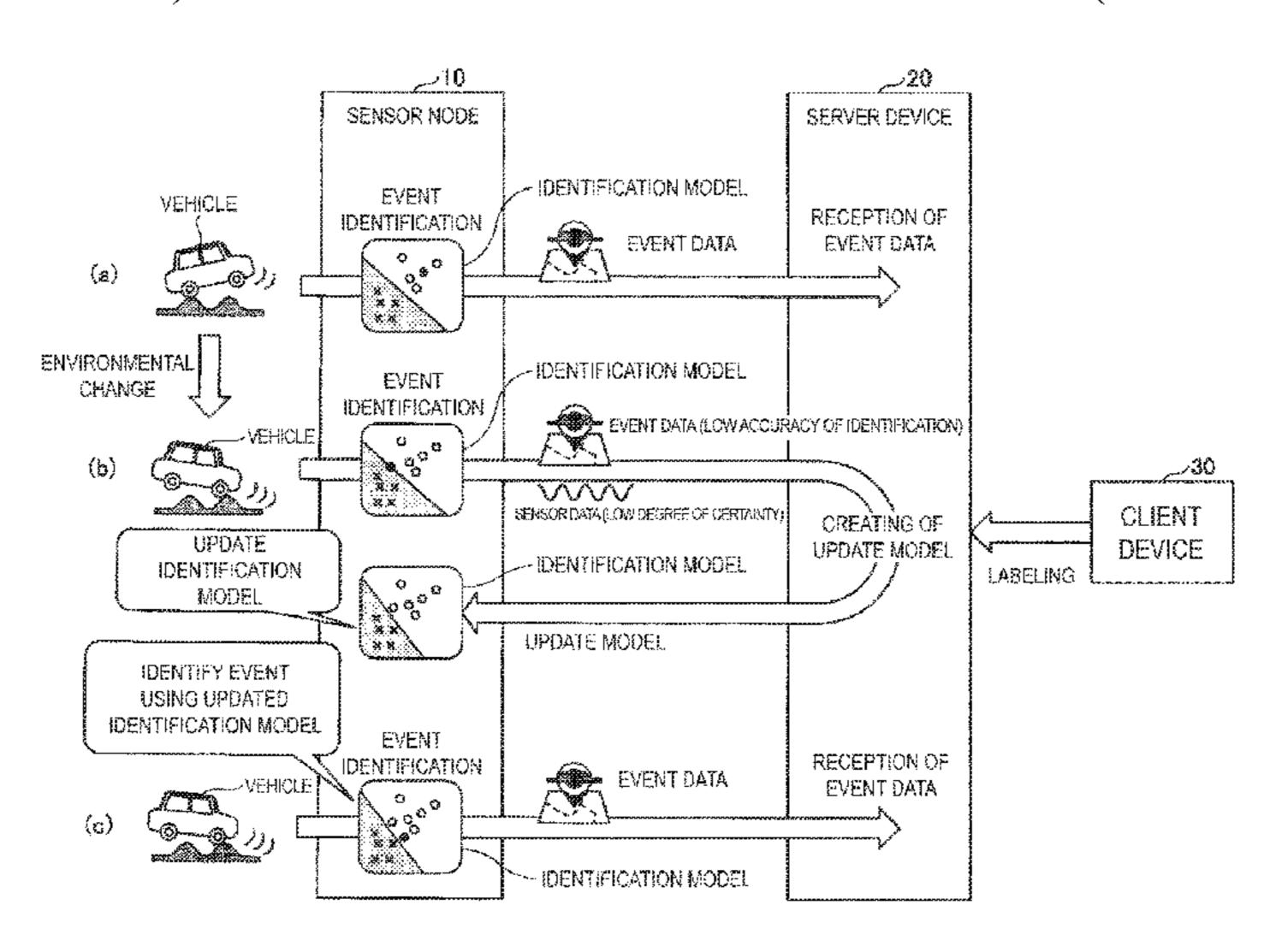
and the degree of certainty of the sensor data are stored in association with each other, and transmit the selected sensor data to the server device.
