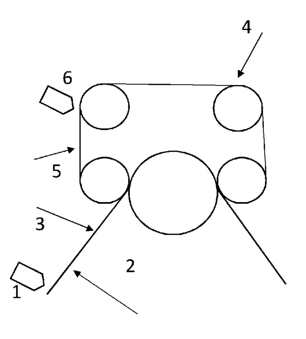
least one calender whereby the coating web is applied to the first side of the web forming the coated paper, paperboard or film. The invention also relates to a paper, paperboard or film produced according to the method.
