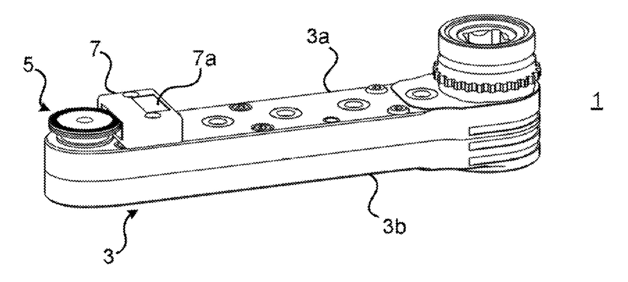
to measure the strain on the socket and thereby obtain a measure of the torque at the output gear wheel.
