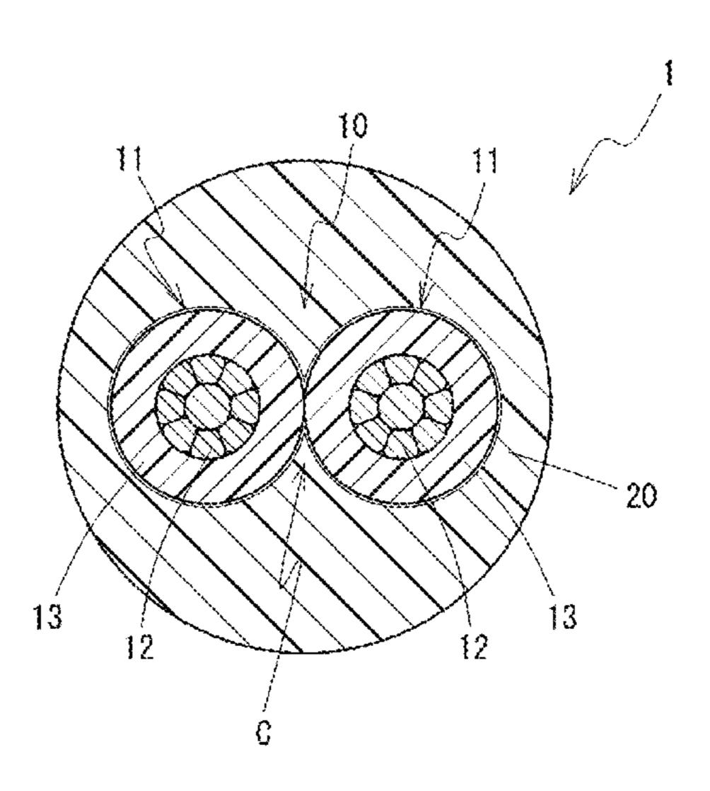
wires and in which transmission characteristics hardly decrease due to a pressure in extrusion-molding a sheath. The signal cable 10 includes a plurality of insulated wires 11 each having a conductor 12 and an insulation coating 13 covering an outer periphery of the conductor 12, and a solid sheath 20 covering an outer periphery of the signal cable 10. A melt flow rate of a constituent material of the sheath 20 measured at 200° and with a load of 2.16 kg is 0.25 g/10 min. or more.
