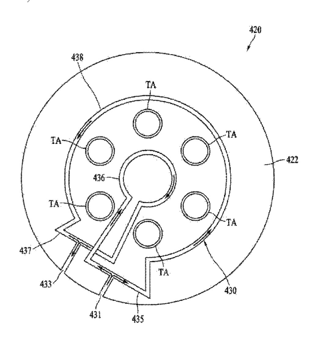
flow path connected to each of the at least one inlet and the at least one outlet, and extending along a second side, different from the first side, of the target area.
