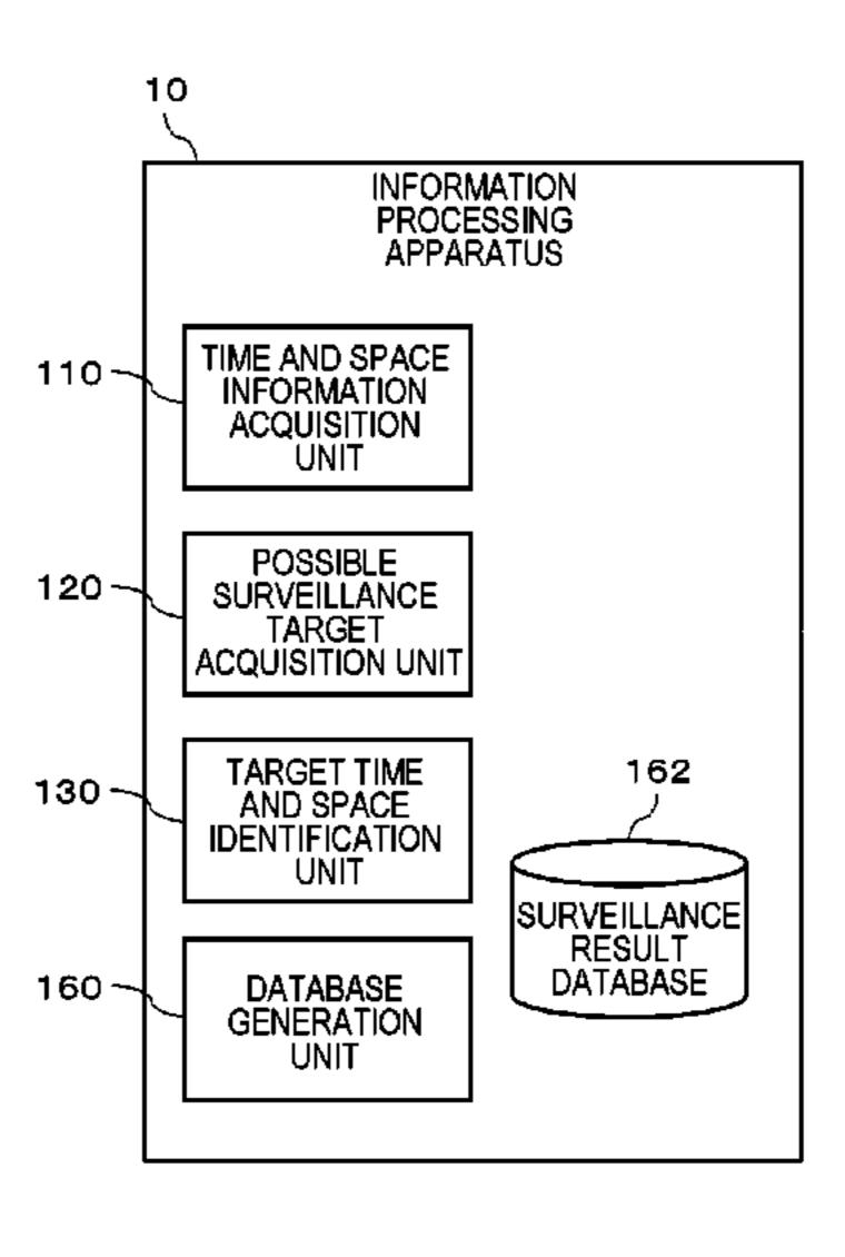
information of a possible surveillance target, and a target time and space identification unit (130) that identifies at least one of a spatial region where surveillance is to be conducted which is at least a portion of the spatial region or a time slot when surveillance is to be conducted, from among the spatial region and the time slot indicated by the high-risk time and space information, on the basis of the information of the possible surveillance target.
