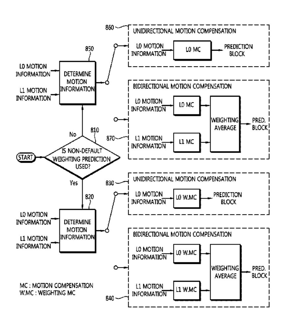
a current block; and generating a prediction block for the current block on the basis of the derived motion information. According to the present invention, computational complexity can be reduced and encoding efficiency can be improved.
