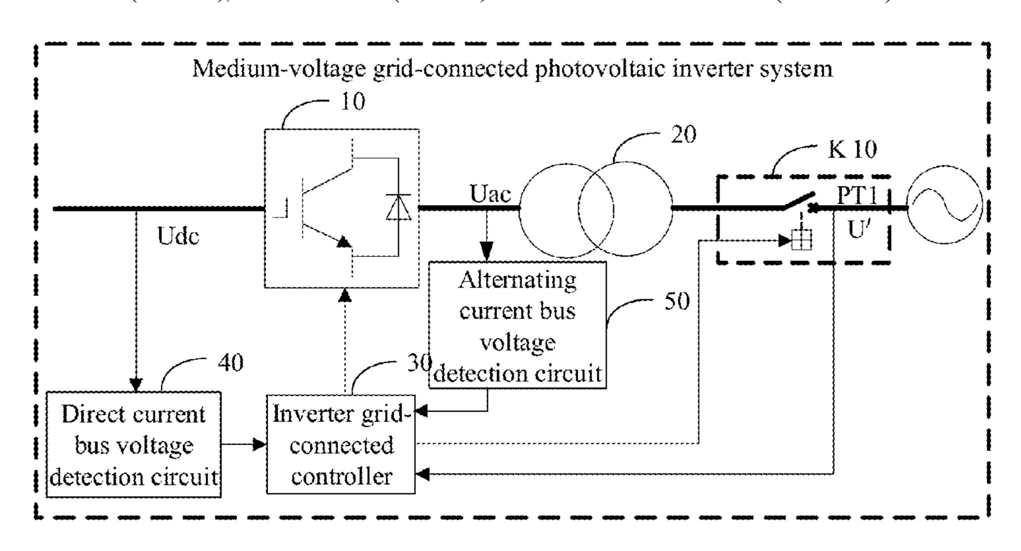
medium-voltage transformer and a line voltage at a side of the medium-voltage grid and generate a grid-connected voltage detection signal. The inverter grid-connected controller is connected to a controlled terminal of the mediumvoltage switch and an output terminal of the voltage sensor.
