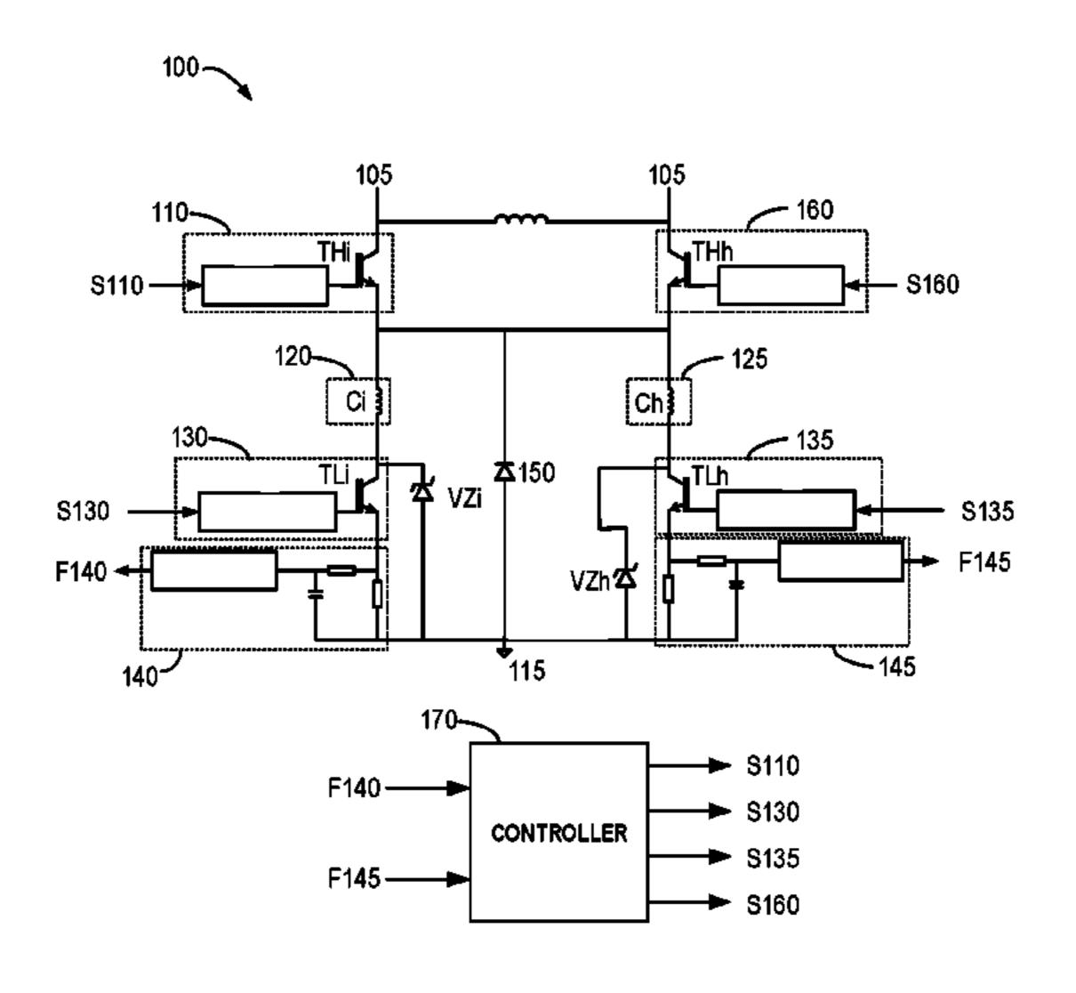
controller is used to control operations of the control units so that in a state that at least one magnetic unit of the first magnetic unit and the second magnetic unit is disconnected from the power supply, a current of the at least one magnetic unit flows through the freewheel unit. According to embodiments of the present disclosure, the contactor may be made more energy-saving, and the operation cost may be reduced.
