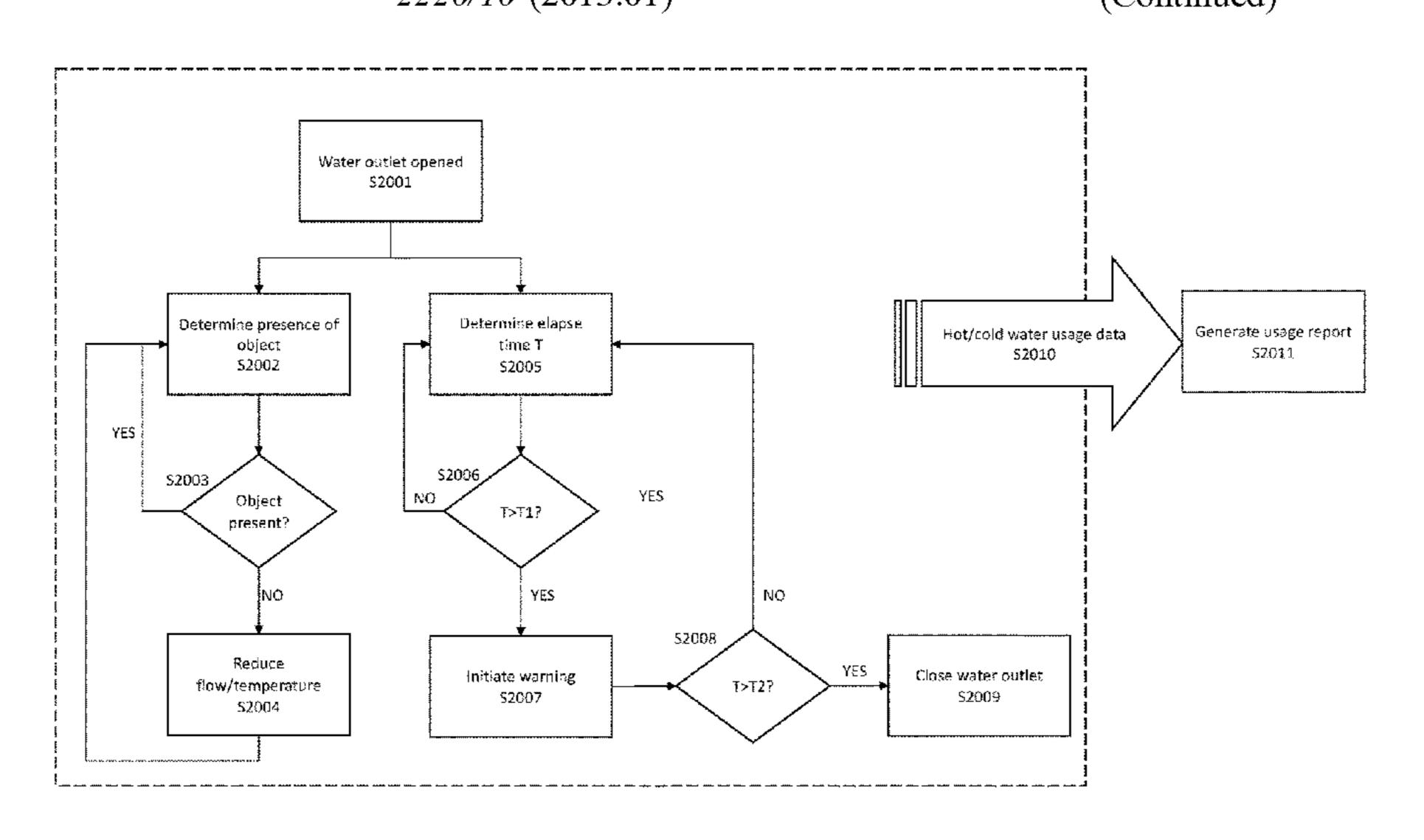
for a user for which the request has been received, upon detecting that the user has opened the water outlet, providing heated water at the first temperature for a first period of time, then reducing the temperature of the heated water from the first temperature to a second temperature lower than the first temperature after the first period of time has elapsed.
