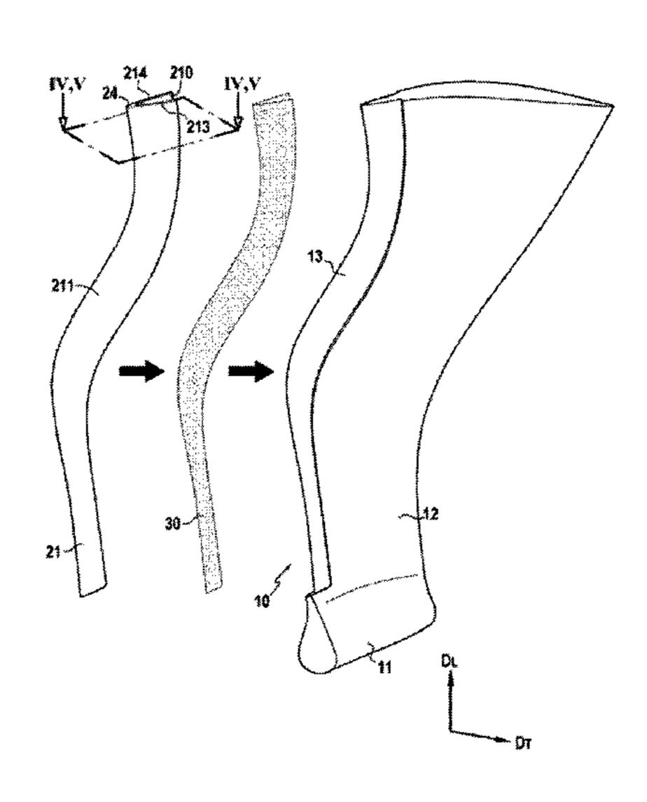
digital model; bonding each manufactured leading edge onto a blade body from the batch of plurality of blade bodies.
