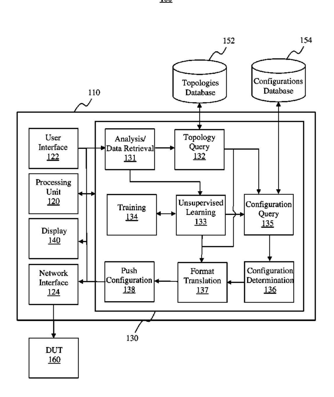
topology or in the predicted network topology in a configurations database; determining design configurations for the network elements of the design network topology from the identified configurations; translating the design configurations of the network elements to a standard format; and pushing the translated design configurations to actual network elements and/or virtual network elements corresponding to the network elements.
