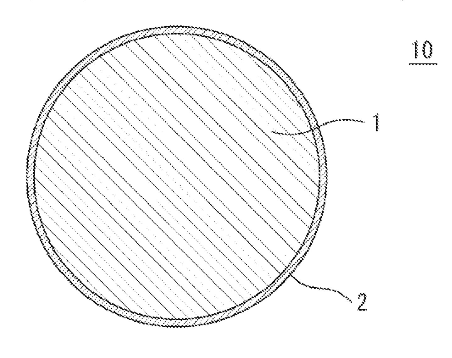
140 nm or less, and has an eluted lithium ion amount of 0.30% by mass or more and 1.00% by mass or less. The coating layer is a composite oxide containing Li and at least one element.
