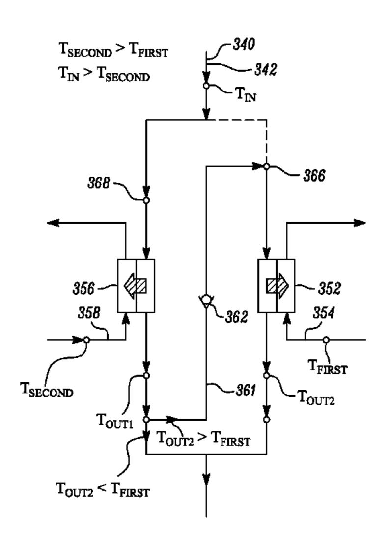
waste heat energy from the first heat transfer fluid is transferred to a first dissipation medium, in dependence on a temperature of the first heat transfer fluid entering the first heat exchanger module, a temperature of the first heat dissipation medium, and a temperature of the second heat dissipation medium.
