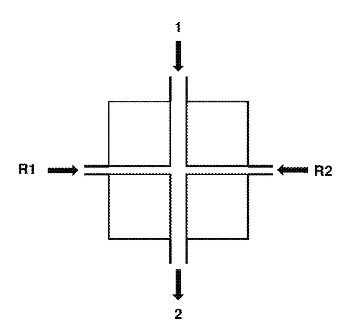
the precondensate from step (a) and the ammonia are each injected by means of a nozzle into a reactor space enclosed by a reactor housing onto a common collision point.
