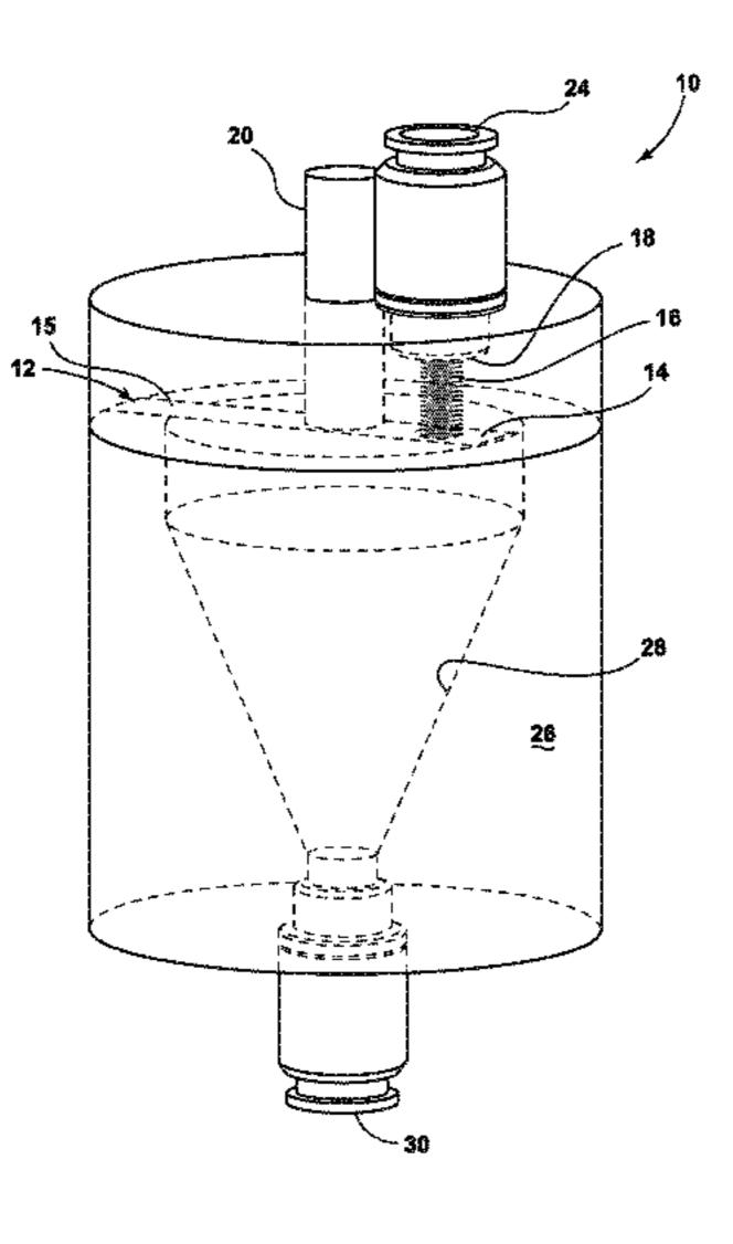
powder material outlet port and includes internal features for smooth travel of metal powder material particles.
