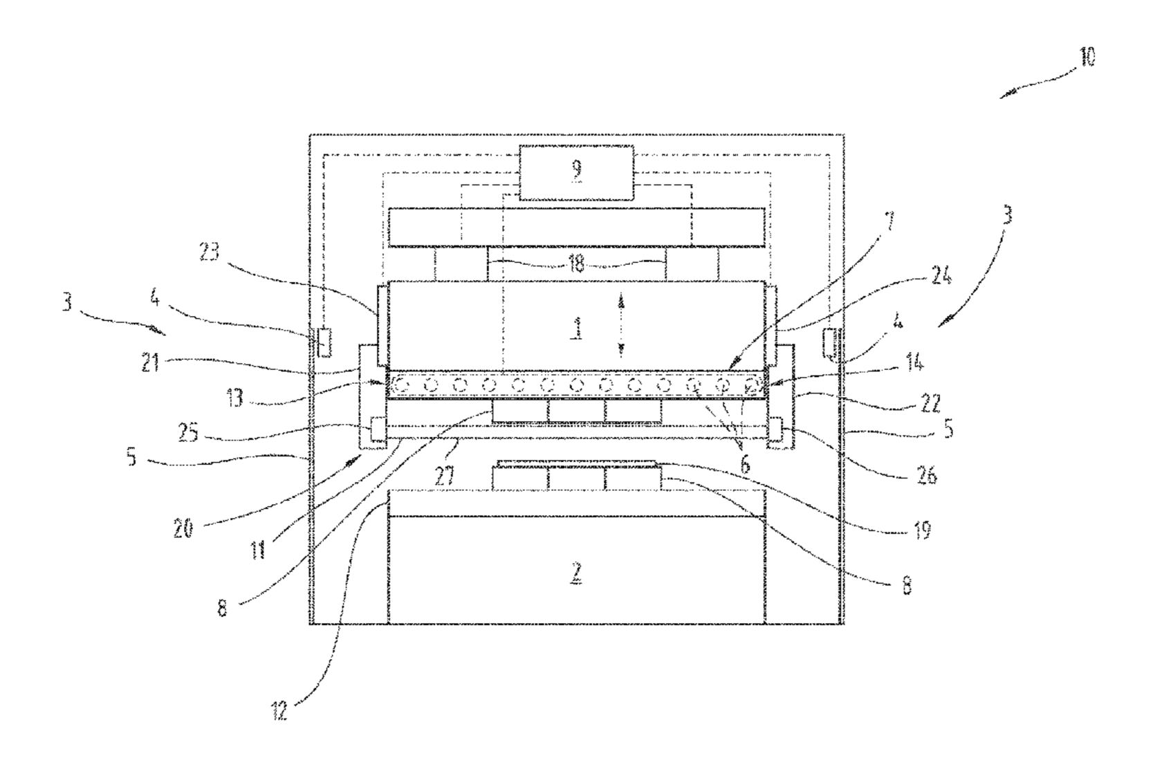
wherein the first mount (21) is arranged on a first side of the first platform (1) and is adjustable relative to the first platform (1) by a first adjustment drive (23),
