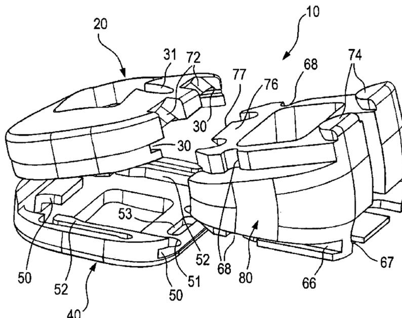
second inter-engaging formation upon insertion of the core component between the superior and inferior components.
