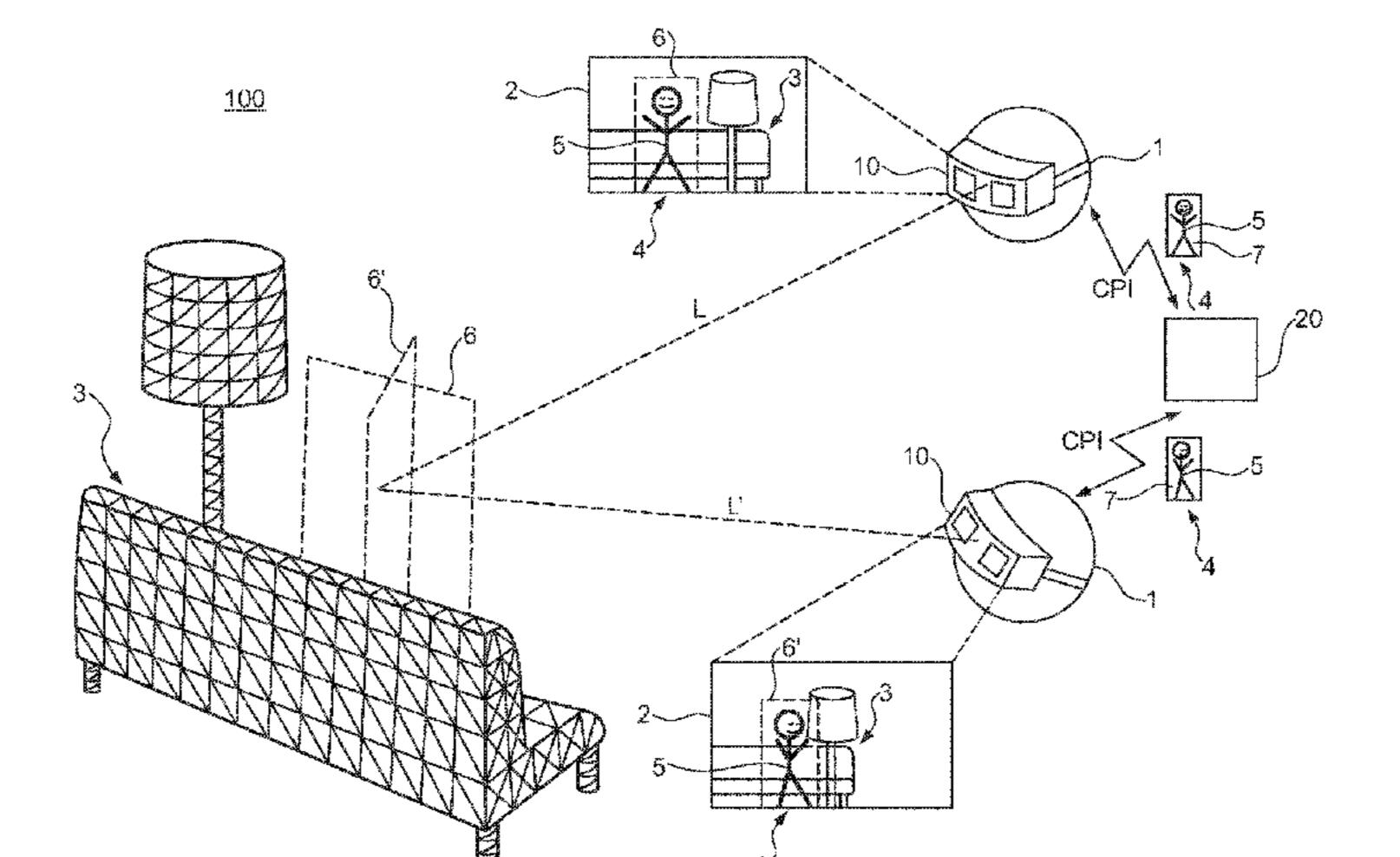
The method further includes receiving a rendered view of the volumetric video object that has been rendered in accordance with the CPI from the remote server. The method also includes augmenting the view of the real-world environment by at least mapping the rendered view of the volumetric video object onto a planar mapping surface arranged according to the desired position of the volumetric video object.
