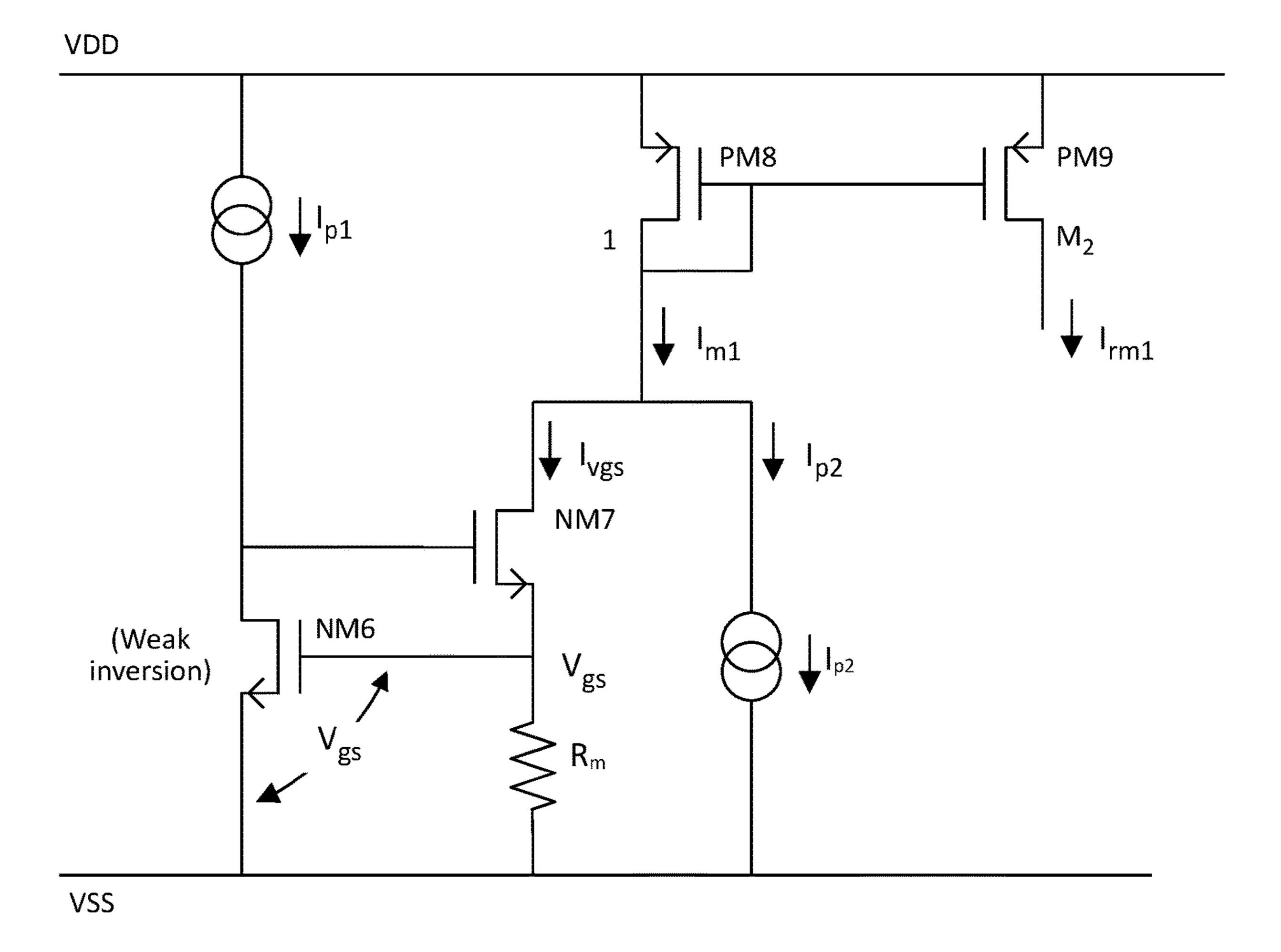
FIG. 7 – MOS-based current reference source
