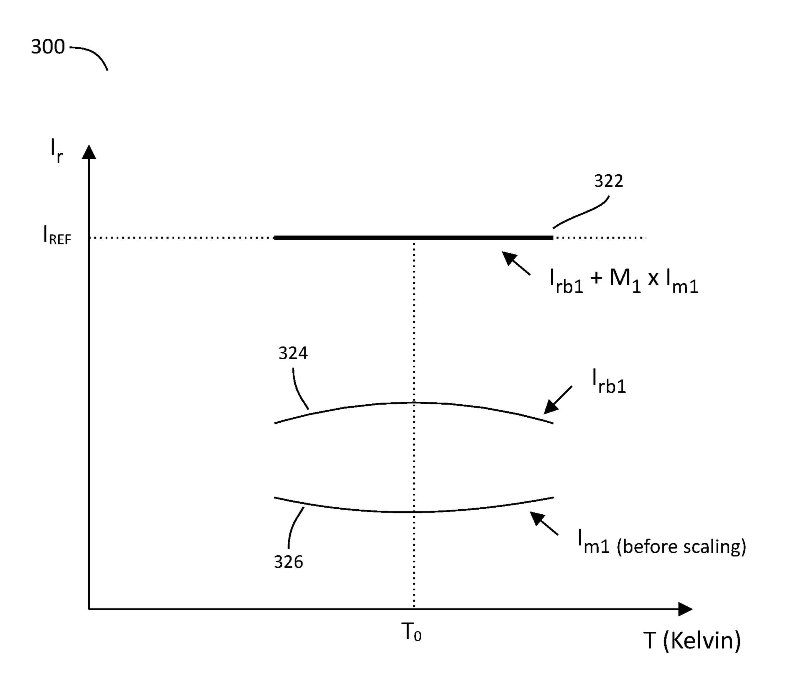
FIG. 3 – Currents versus temperature
