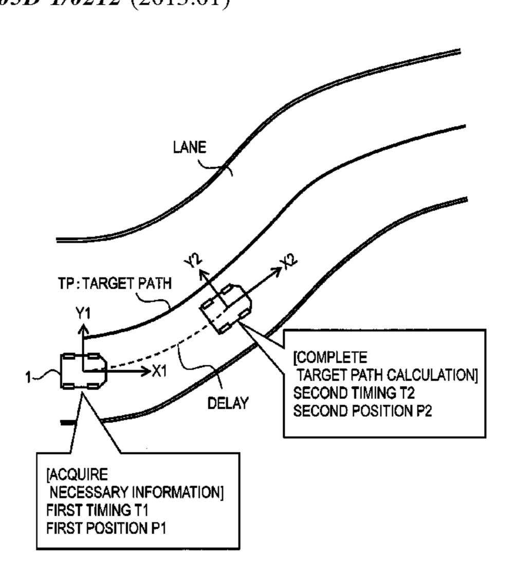
system. The autonomous driving system uses the second target path as the target path to perform the vehicle travel control.
