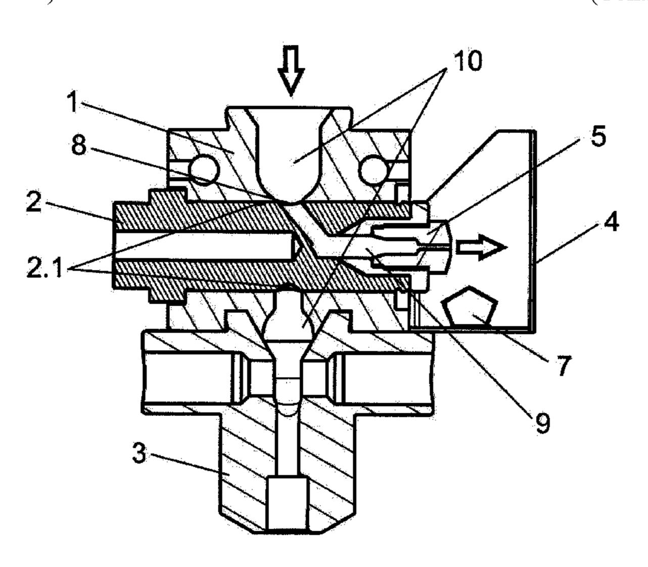
depending on the angular positions of the piston, material can be conveyed through the at least one groove to the outlet nozzle or through the hole to the bypass nozzle.
