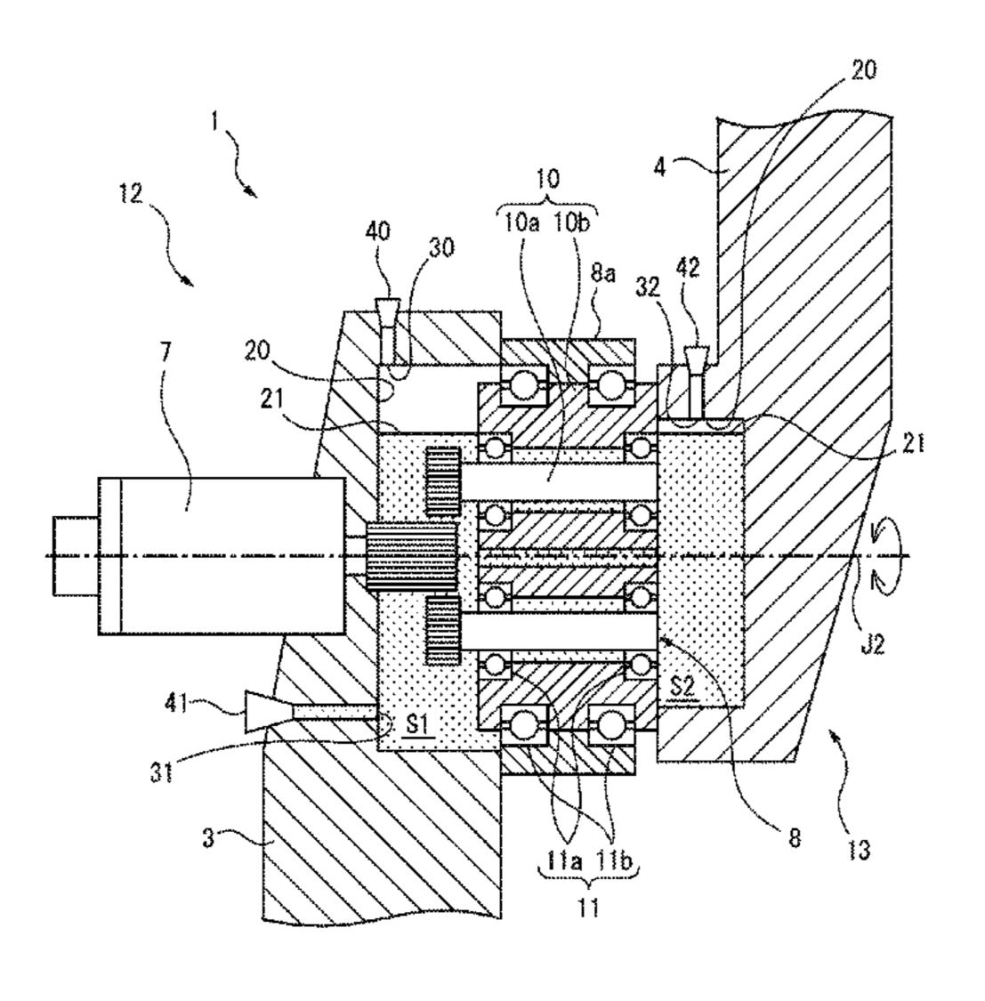
introduction hole; and when the lubricant is drained, the two through-holes are open as ventilation holes, and the remaining through-hole (for example, a through-hole) is open as a lubricant drainage hole.
