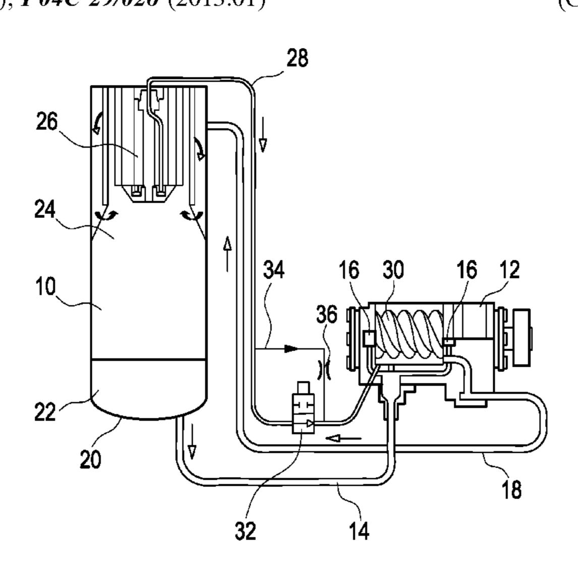
drawn via the scavenge line into the vacuum pump. In accordance to the present invention a valve is disposed in the scavenge line to selectively separate the air filter from the vacuum pump.
