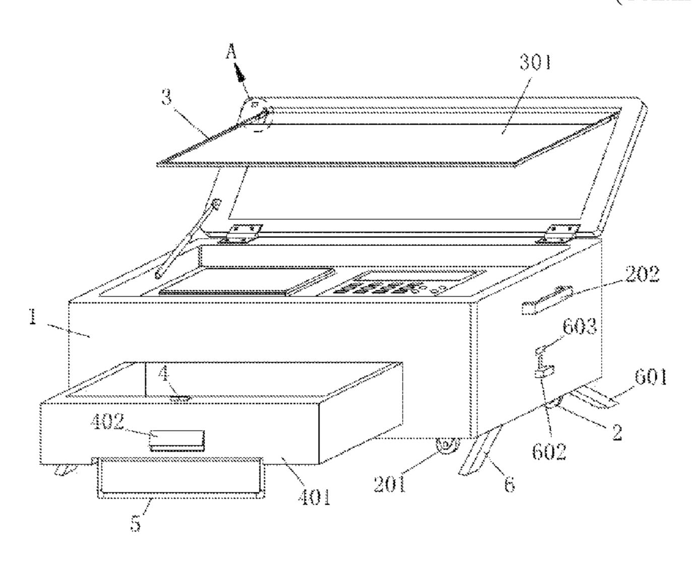
storage box body, a shielding structure for shielding sunlight is connected to the storage box body, an accommodating structure for accommodating an article is connected to the storage box body, a support structure for supporting is connected to the accommodating structure, and a placing structure for placing is connected to the storage box body.
