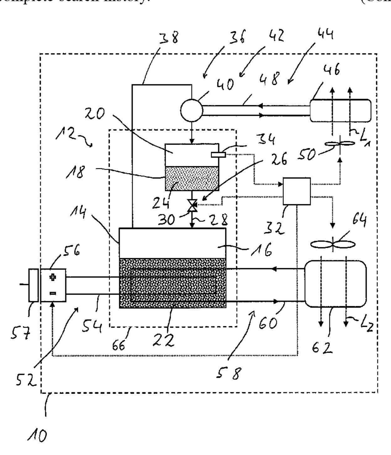
A heating unit (52) heats the first reactant or/and heats the reaction product contained in the reaction space. A reactant-recirculating device (36) recirculates second reactant from the reaction space into the reactant storage space.
