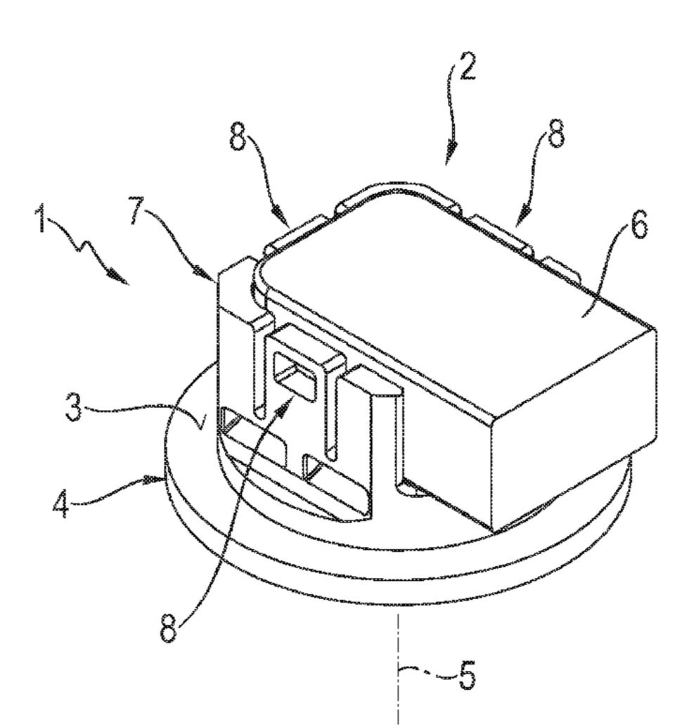
(1, 28) has a receptacle (2, 29) which is made of a plastic material and is injection-molded onto one side (3) of the closure element (1).
