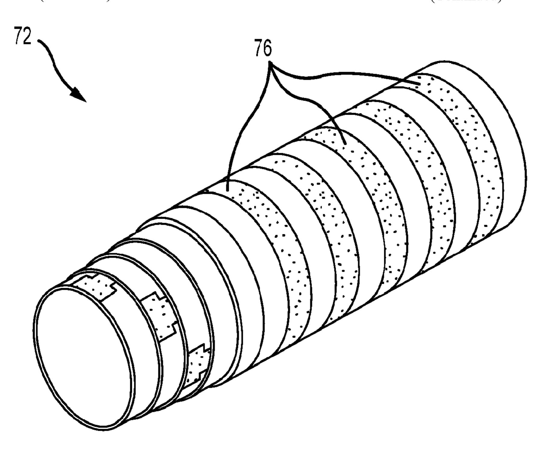
embodiments, the plurality of non-conductive tubular substrates includes a plurality of non-conductive, unitary molded cylinders.
