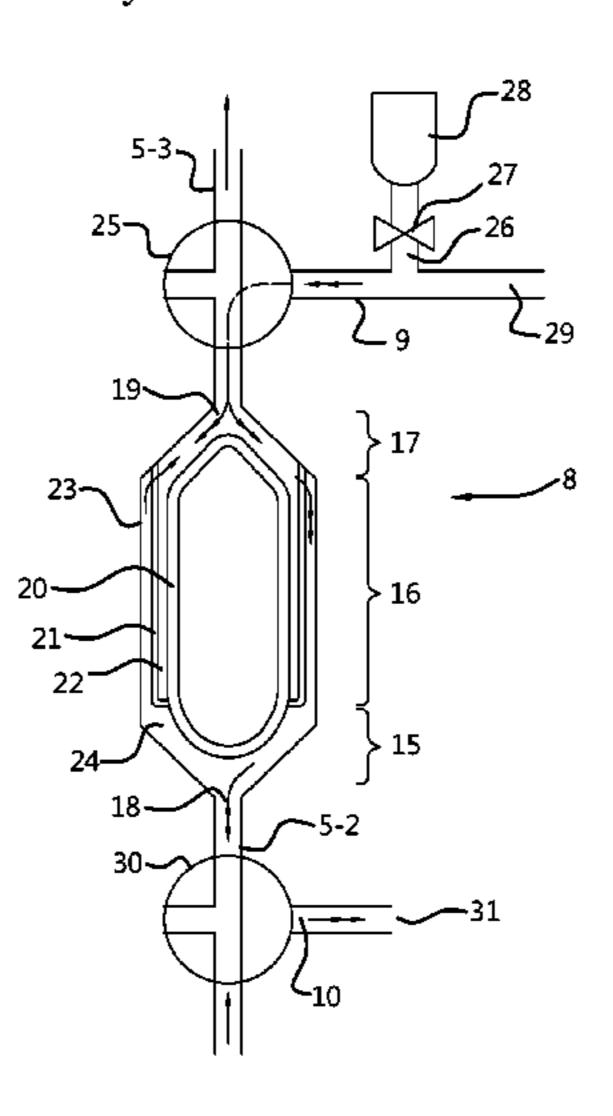
part, viewed in a direction towards the second liquid connection, does not extend beyond the filter plate. In this way, the stream of cleaning liquid, supplied from above, can develop beyond the top part to form a more turbulent stream parallel to the cylindrical part, and thus a more thorough cleaning of, in particular, the upper filter holes. In addition, a milking device including this milk filter is provided.
