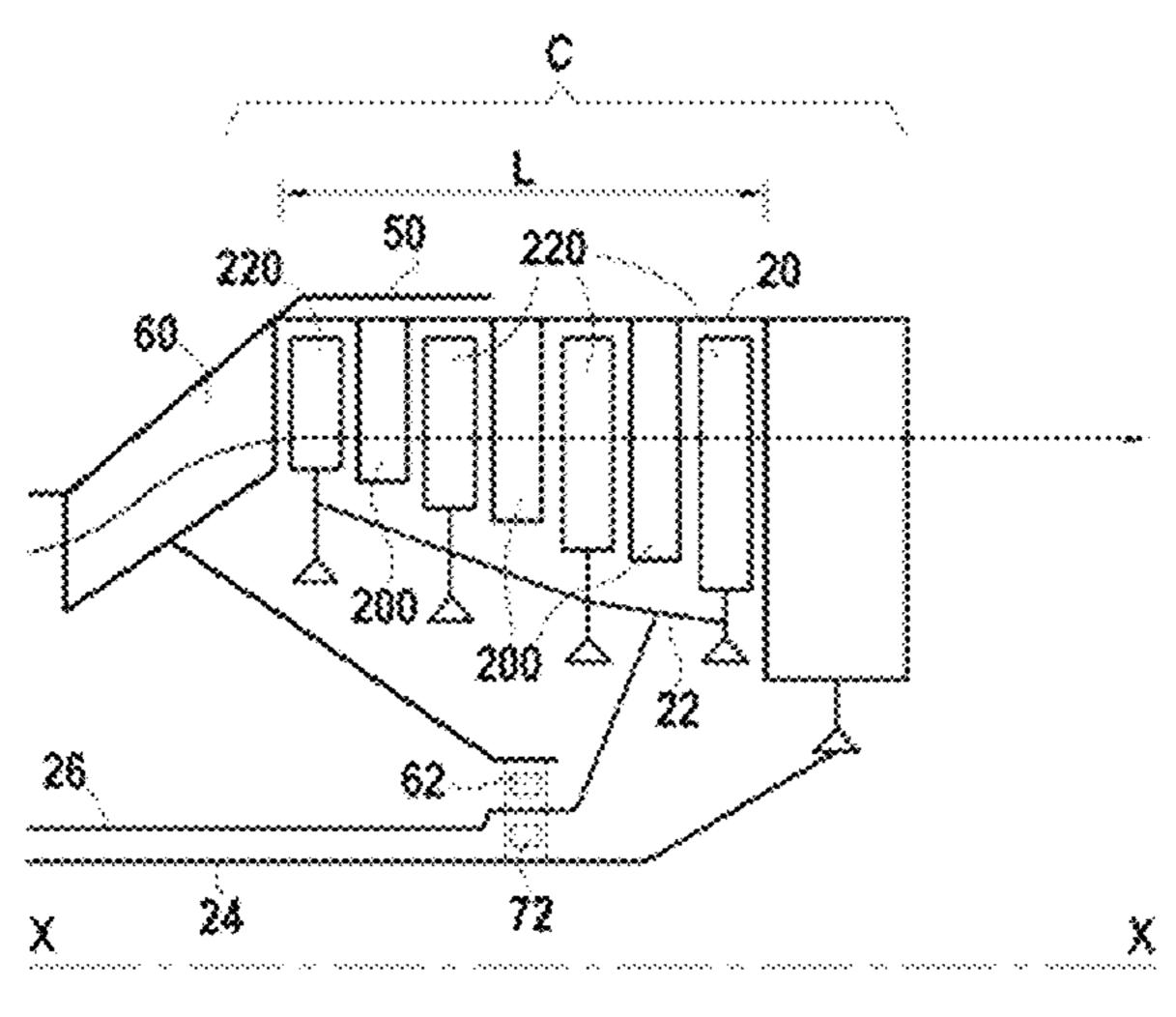
and the second shaft is guided in rotation by a second bearing disposed between the second shaft and said upstream casing of the turbine.
