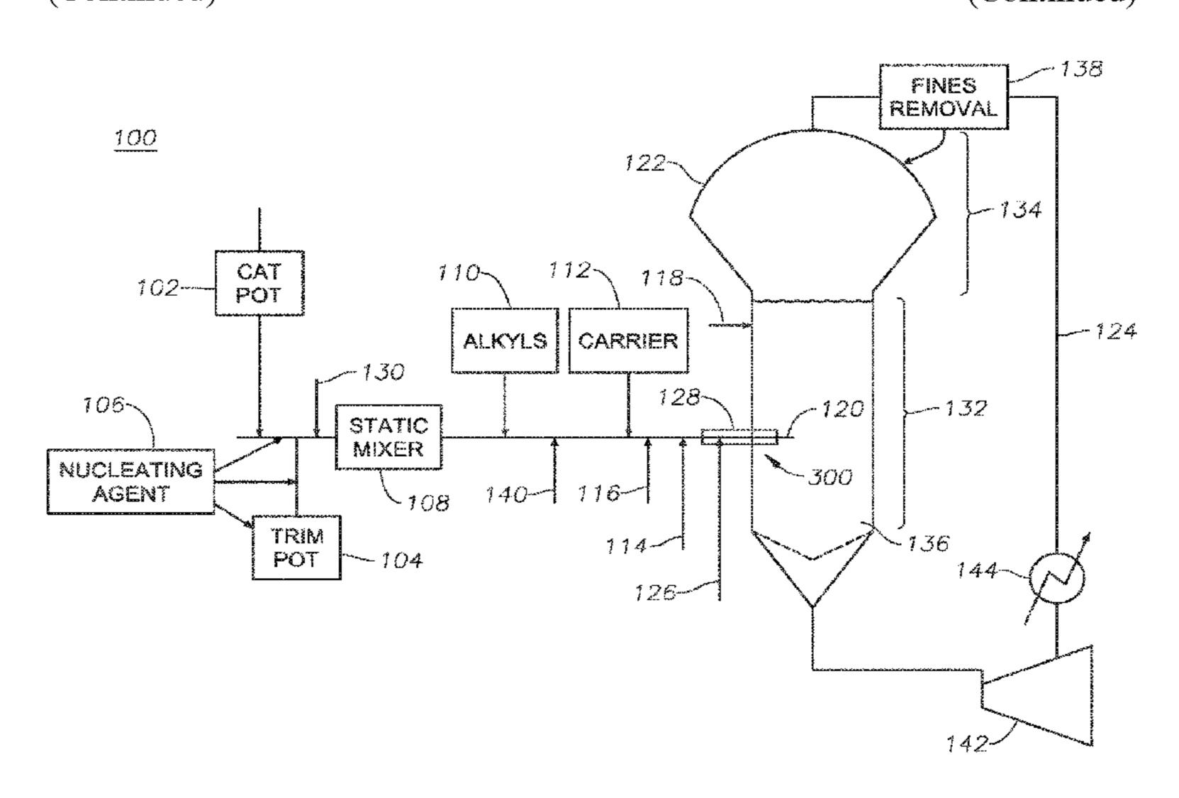
comprises a mol ratio of the third catalyst to the second catalyst to the first catalyst of from 10:35:55 to 60:15:25, such as 30:20:30; introducing the third composition from the line into a gas-phase fluidized bed reactor; exposing the third composition to polymerization conditions; and obtaining a polyolefin.
