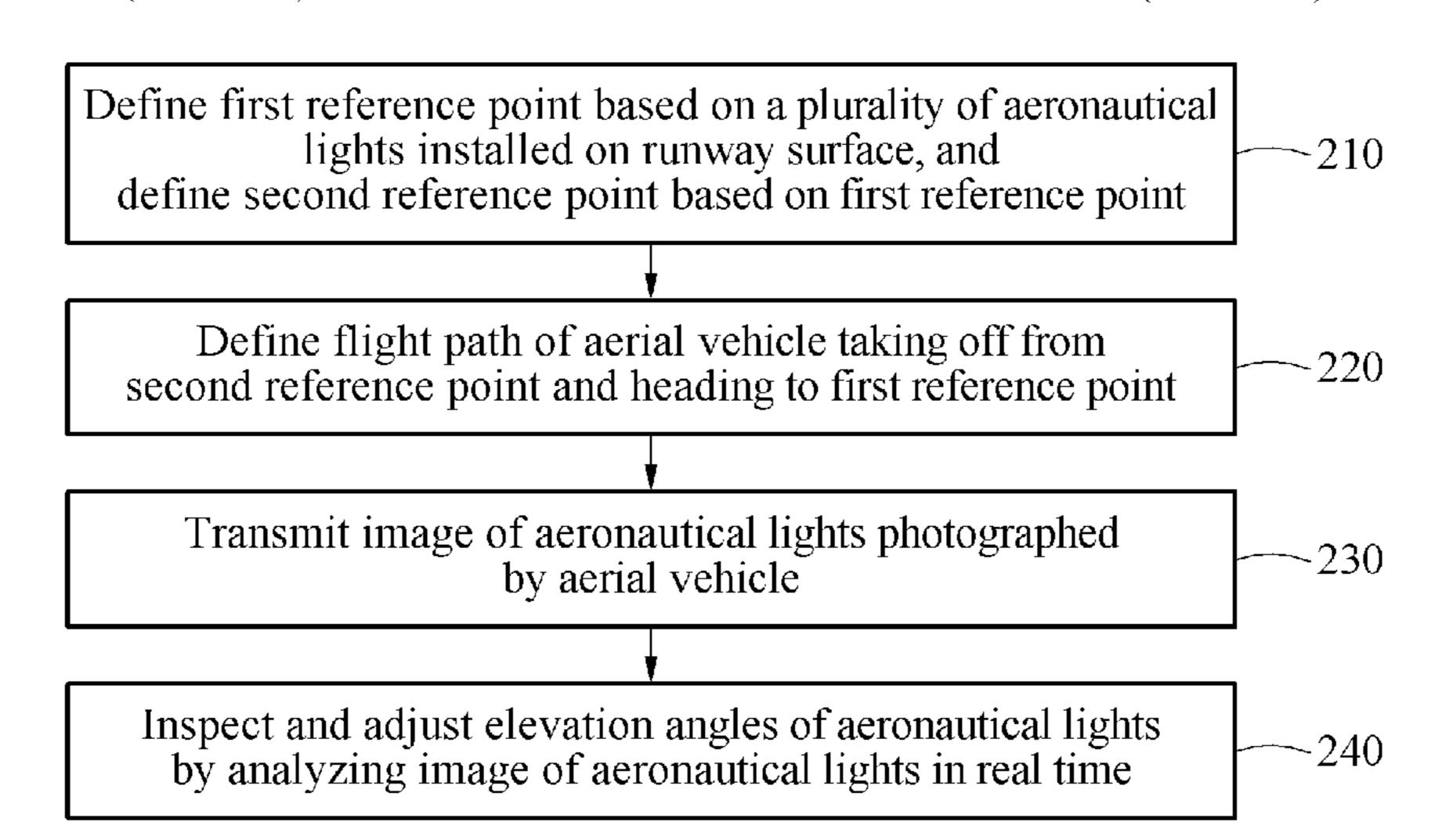
reference point, transmitting, to the ground, an image of the aeronautical lights photographed by the aerial vehicle, and inspecting and adjusting elevation angles of the aeronautical lights by analyzing the image of the aeronautical lights in real time.
