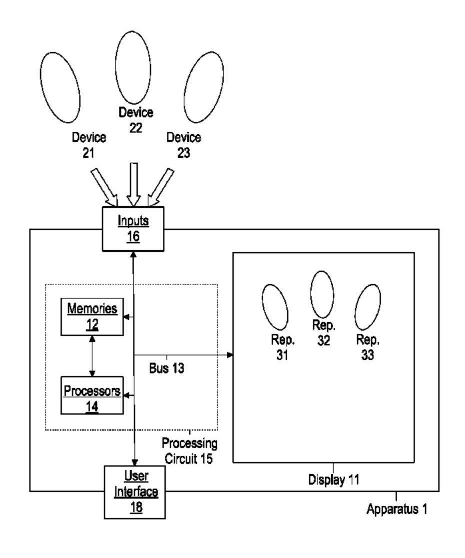
(31-39) via the sequence. Alternatively the triggering procedures may define unique codes to be allocated to the representations (31-39) and to be provided to the devices (21-29), with the identifying information further comprising the codes. The processor (14) can then link the identifiers and the representations (31-39) via the codes.
