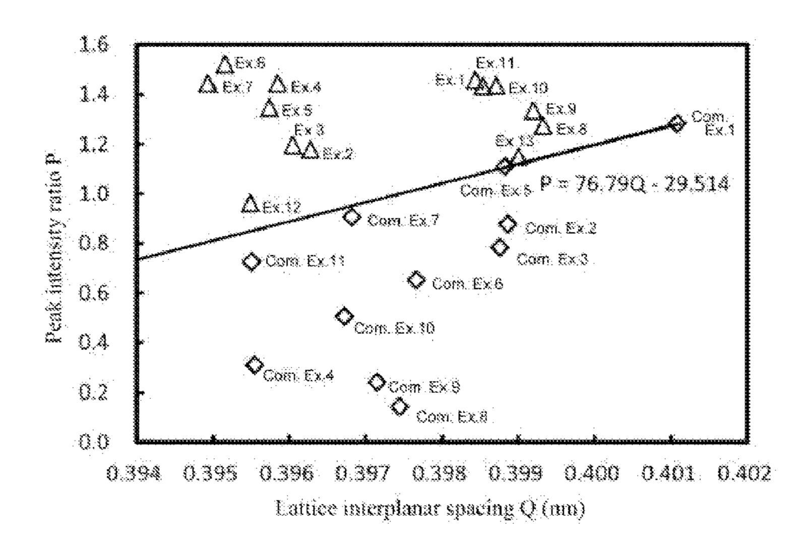
the beta zeolite, the α-alumina being the standard substance 674a distributed by the American National Institute of Standards and Technology, and Q represents a lattice interplanar spacing of the main peak of the beta zeolite observed by X-ray diffraction measurement. It is preferable that the formula (1) above is satisfied in a range in which Q is from 0.3940 to 0.4000 nm.
