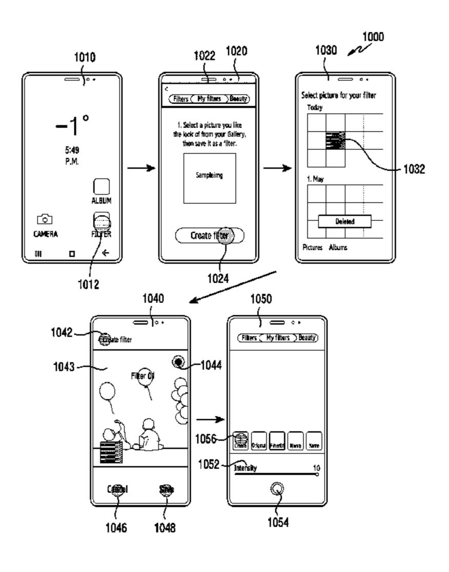
filter may include the function derived by comparing the first image and the second image, the coefficients of the function, and a color lookup table generated on the basis of the derived function. The processor stores the generated color filter in the memory and generates the fourth image by applying the stored color filter to the third image.
