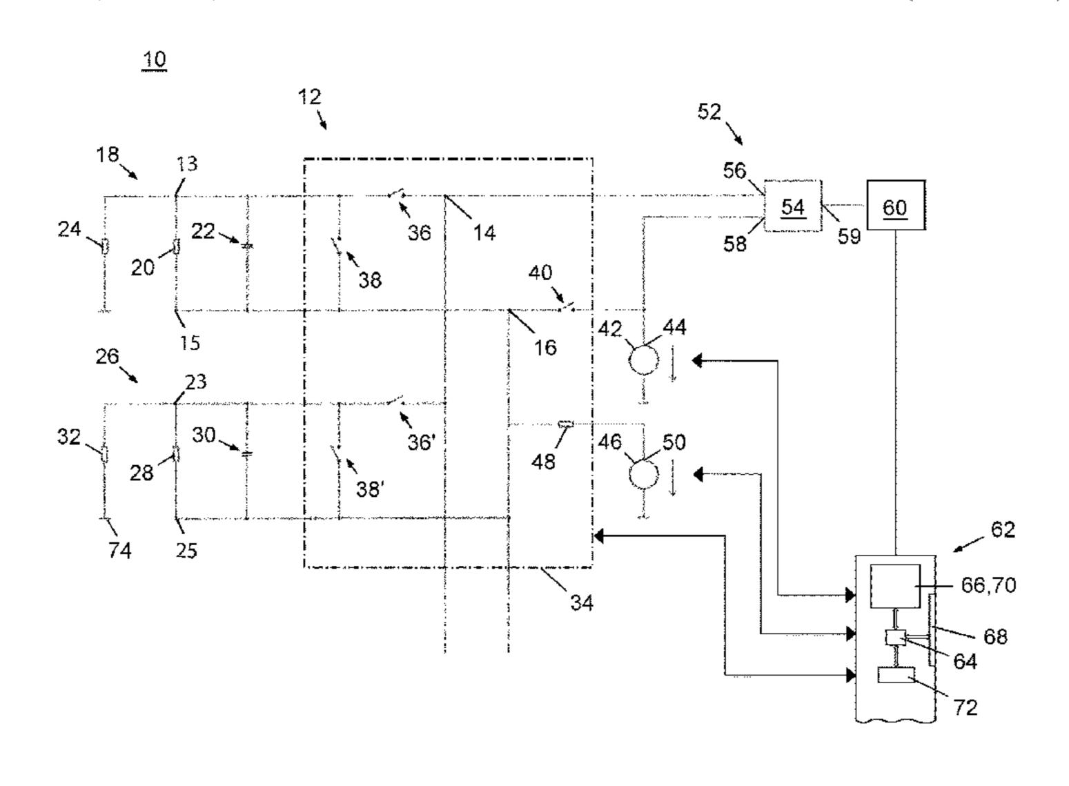
lable manner. A current measurement circuit is connected with a signal input port to the common sense node and with a reference input port to the output port of the measurement signal voltage source.
