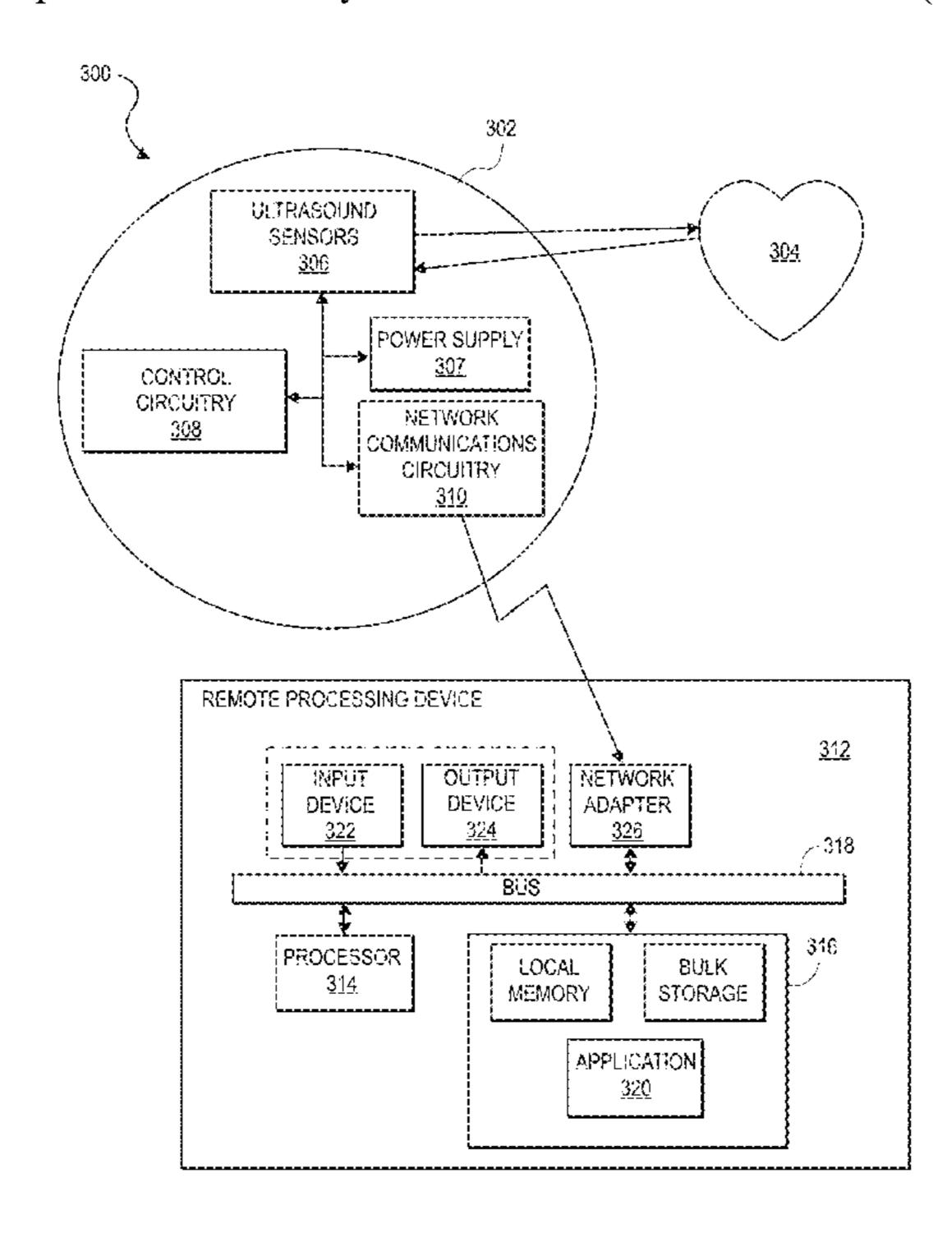
signals based on the beam reflection indicative of a distance of the heart from the ultrasound sensor; and a processing system for receiving the data signals from the control circuitry and processing the data signals to track movement of the subject's heart over time, wherein changes in the movement correlate to the subject's heart condition.
