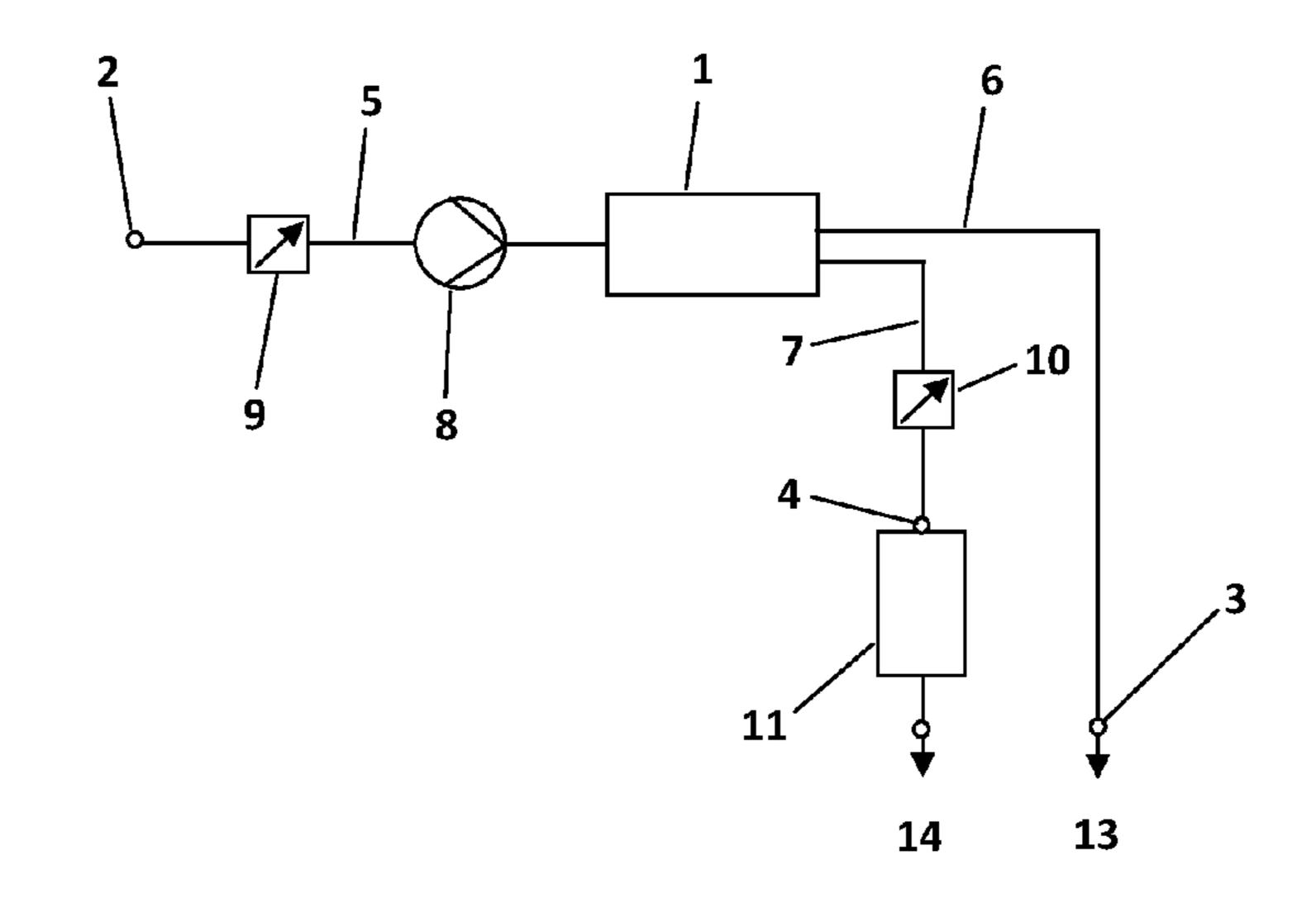
arranged in the cold water path or in the first hot water path, and at least one second flow meter that is arranged in the at least one second hot water path. A method of determining hot water amounts dispensed by a beverage maker and/or hot water amounts used for beverage preparation is also disclosed.
