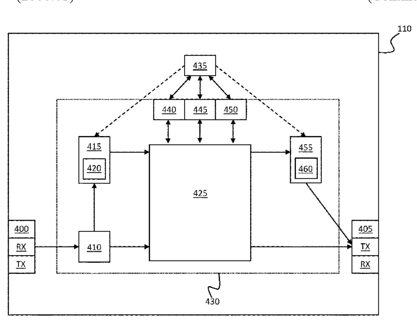
to the decryption unit. The decryption unit is configured to decrypt the encrypted portion of the telegram with a key, and to forward the encrypted portion to the processing unit for processing. If an unencrypted telegram is present at the input port, the receiving logic is configured to forward the unencrypted telegram to the processing unit for processing.
